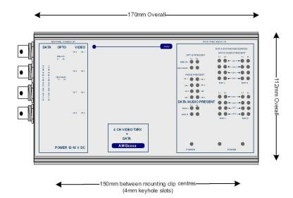
The **AMG4647A-SF** is a standalone four channel video transmit unit designed to transmit 4 video signals and transmit and receive up to 8 data or audio signals over one Multimode fibre. The 8 data/audio channel interfaces, whether RS232, RS422, RS485, 20mA, TTL, Contact Closure, Lonworks or Audio, are defined at manufacture by the addition of daughter boards fitted onto the Data Expansion Board A.
